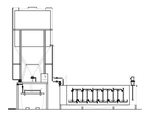
PAINT STRIPPING TANK WITH SLUDGE REMOVING SYSTEM
